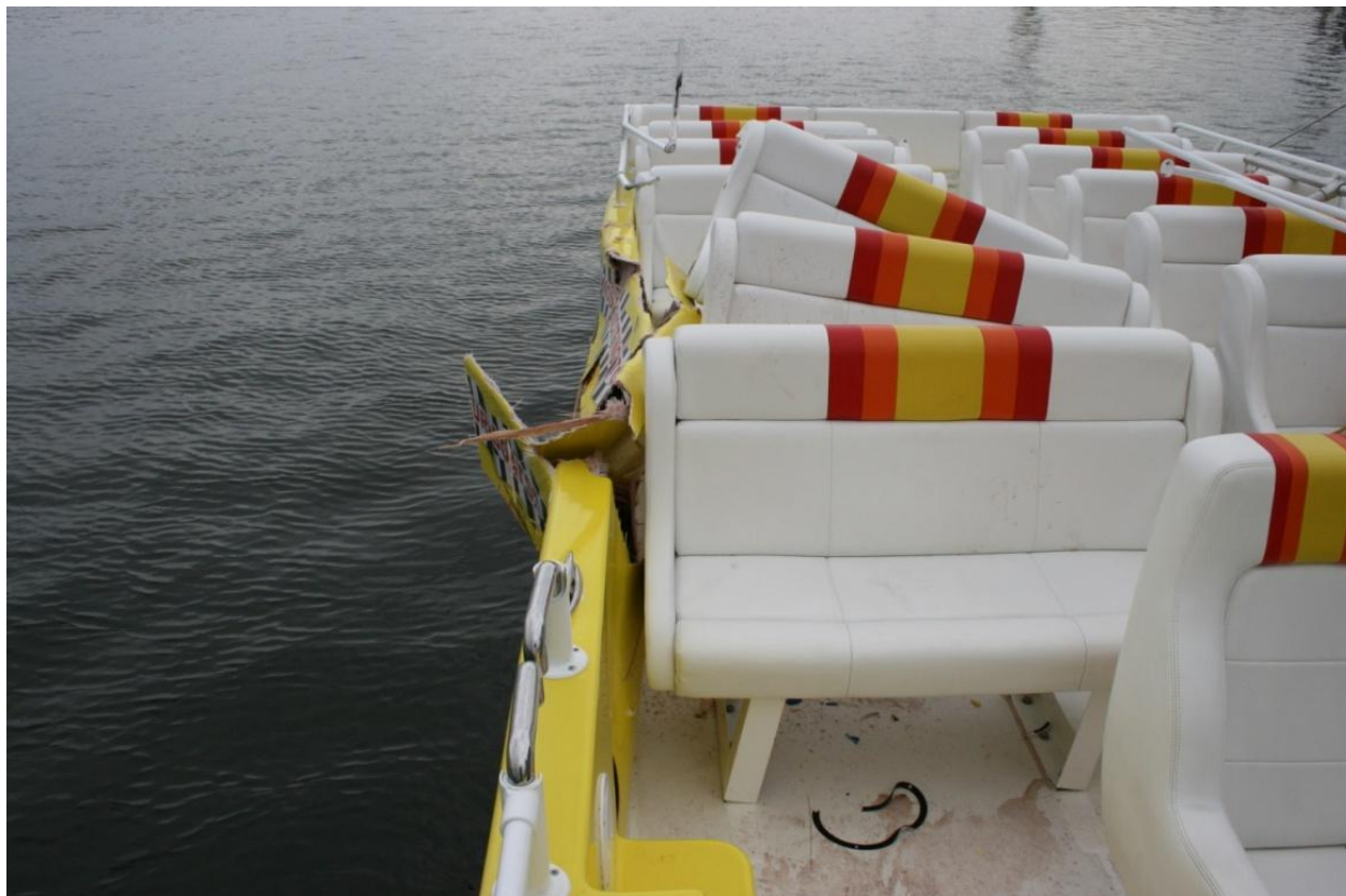
Figure 5. Damage to Thriller 09 starboard side, looking aft from the bridge.
