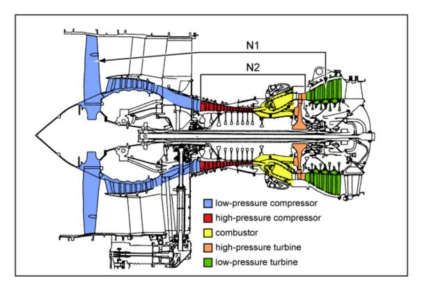
Figure 4. Cutaway of a turbofan engine showing the LPC, HPC, combustor, HPT, and LPT.
