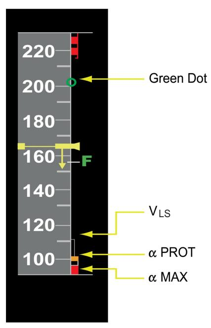
**Figure 3.** The A320 airspeed scale, including select characteristics and protection speeds.
