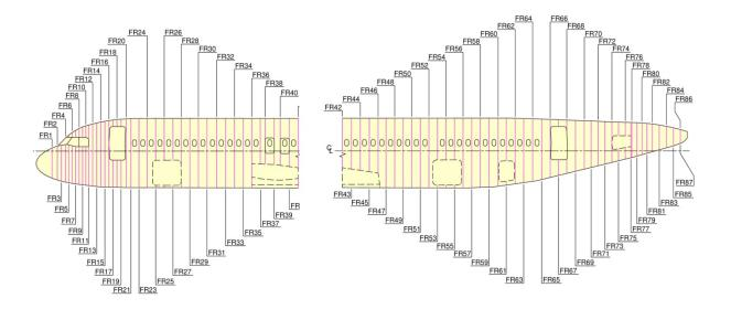
**Figure 6.** Diagram showing the A320 fuselage frame locations.
