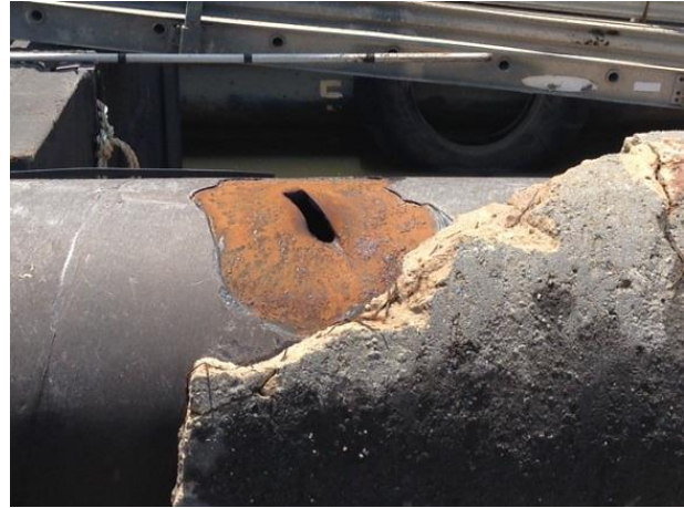
Left, the Shanon E. Settoon's damaged propeller blade during postaccident survey; right, the damaged pipeline and its protective casing. (Photos by the Coast Guard)
