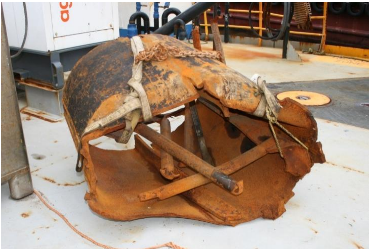
Figure 11. A section of Trinity II 's fractured stern leg.
