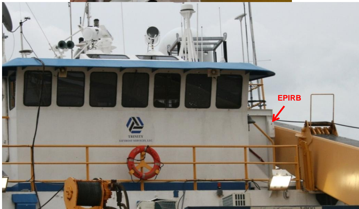
Figure 7. The Trinity II 's EPIRB during postaccident examination, and the EPIRB's location on the portside bulkhead just outside the wheelhouse.
