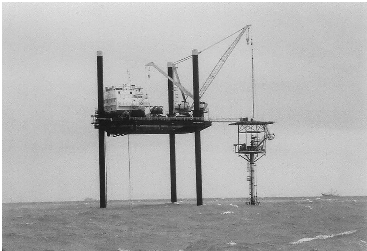
Figure 3. File photo, provided by Trinity Liftboats, showing the Trinity II jacked up during operations.
