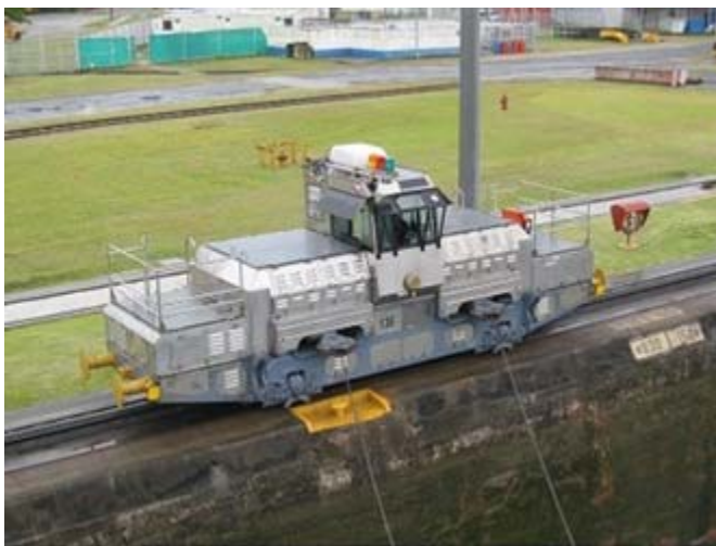
Electric locomotive (mule) used in original locks
